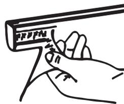
The blind is mounted to the cassette with a Velcro tape, which enables washing it.
