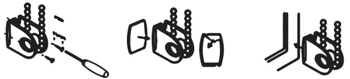
Mounting with screws to the wall. Installation with adhesive tape to the window.
